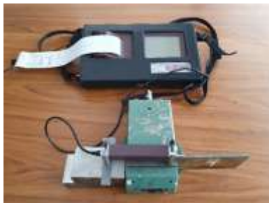
Fig.2. Portable digital roughness meter, positioning the feed unit on the workpiece
